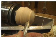
1. The reverse chucked piece is now rounded
