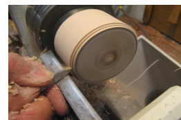
2. Mount the second half and cut a tenon
