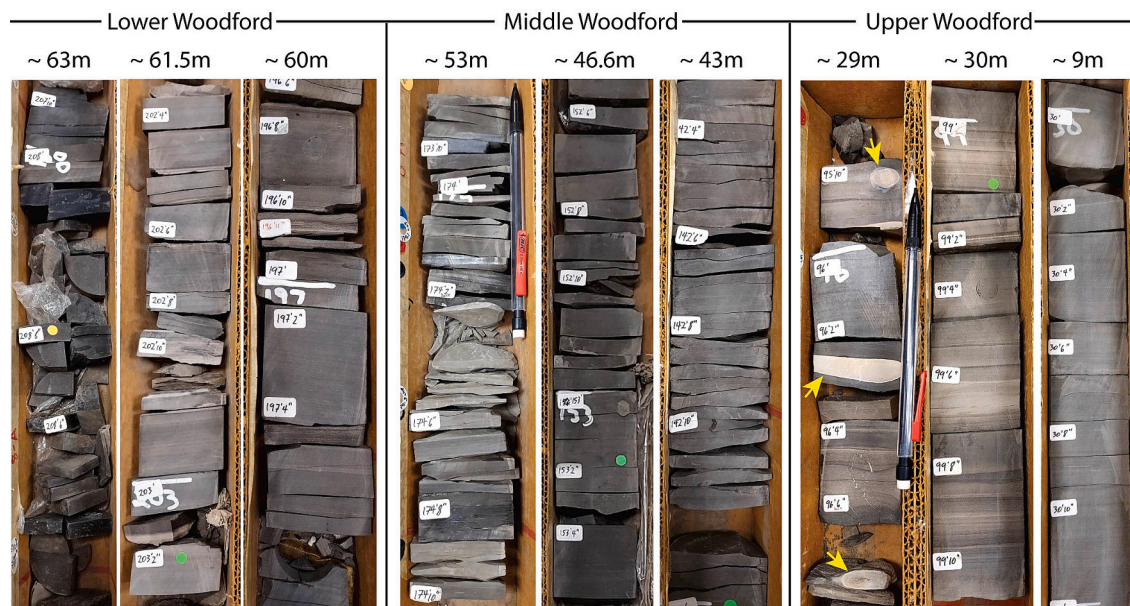
Fig. 3. Lower, middle, and upper Woodford Shale core photos from the northern shelf site, Wyche-1 core. Yellow arrows in the upper Woodford Shale point to phosphate nodules. Core depth tags are measured in feet and inches with a tag every two inches. Approximate depth in meters is posted above each core profile. (For interpretation of the references to colour in this figure legend, the reader is referred to the web version of this article.)
