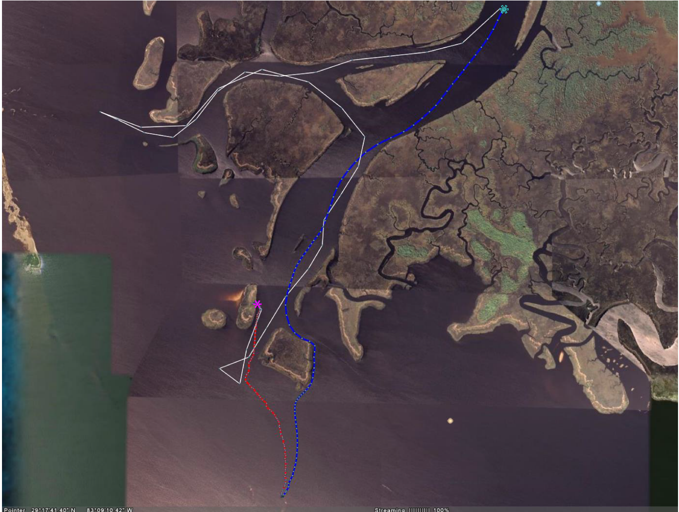
Figure 2: Drifter tracks for deployment at the Suwannee River the 9 th April of 2008. Deployment and recovery sites are indicated with the green and cyan stars, respectively. The white lines indicate the drifter trajectories. Dots represent the 5-minute interpolated positions, and are all blue for an outgoing tide.
